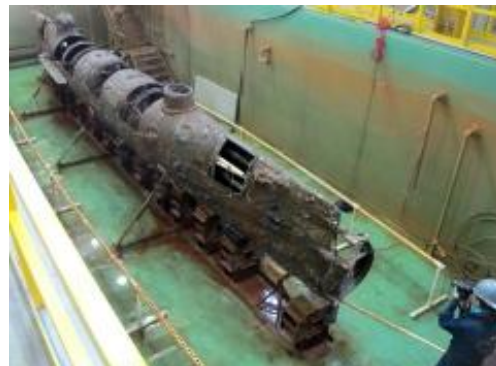
H. L. Hunley, suspended from a crane during its recovery from Charleston Harbor & sitting in a conservation tank after the steel truss that had surrounded it was removed.
