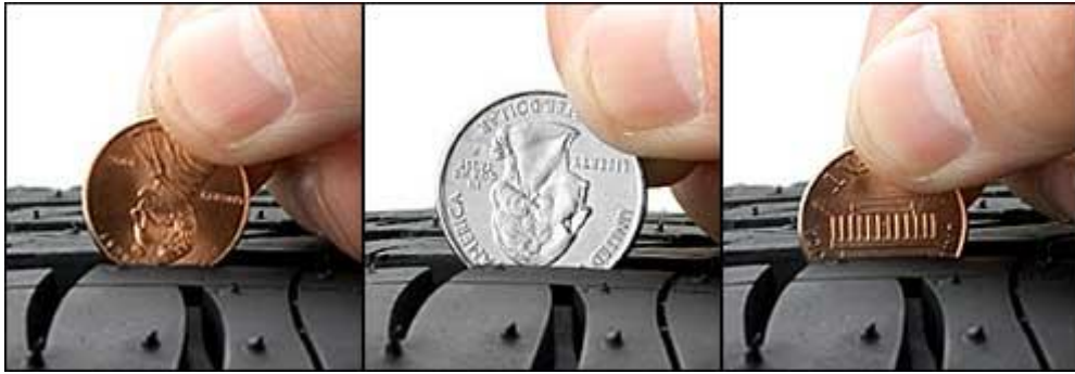
2/32" remaining tread depth 4/32" remaining tread depth 6/32" remaining tread depth
