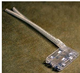
The seven-millimeter-long cuff electrode
